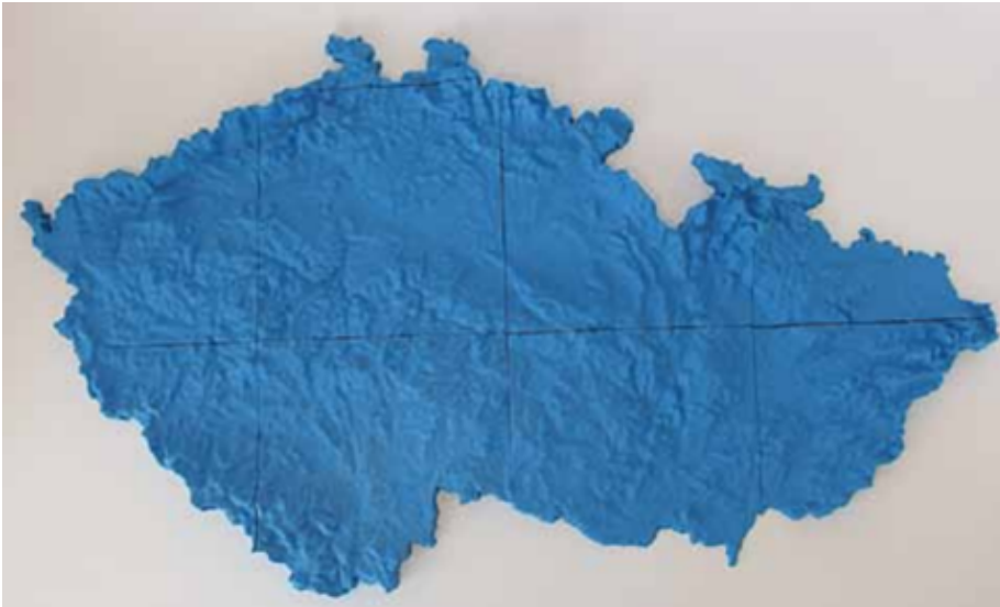
Fig. 19: The digital model of the relief of the Czech Republic printed on a Prusa i3 3D printer. Model size 700 × 400 × 32 mm. Source: Brus and Barviř 2016
